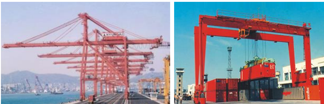
Figure 10.5: Rail Mounted Quay Cranes (RMQC) & Rubber Tyre Gantry Crane( RTGC)
