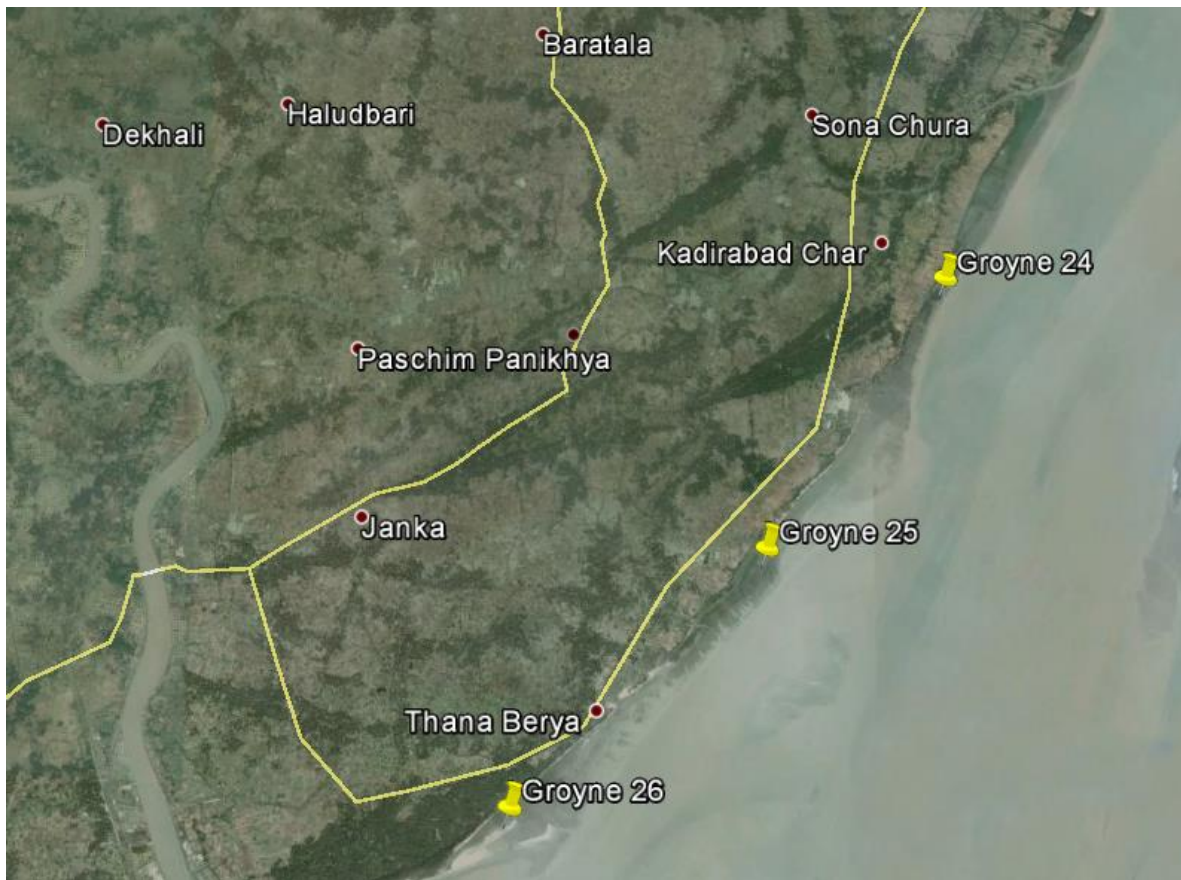
Figure 2.3: Area north of Rosulpur River reclaimed by sand due to Groynes 25 & 26
